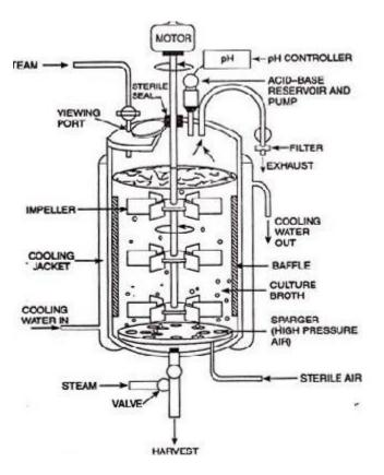
DIAGRAMATIC DESIGN OF A FERMENTOR WITH CONTROLS
